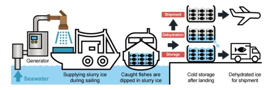
The use of slurry ice is the best option for chilling fish on board small and medium size fishing vessels
