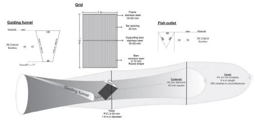
Fig 1. Shematic diagram of sorting system used in experiment (Aydin et al., 2011)
